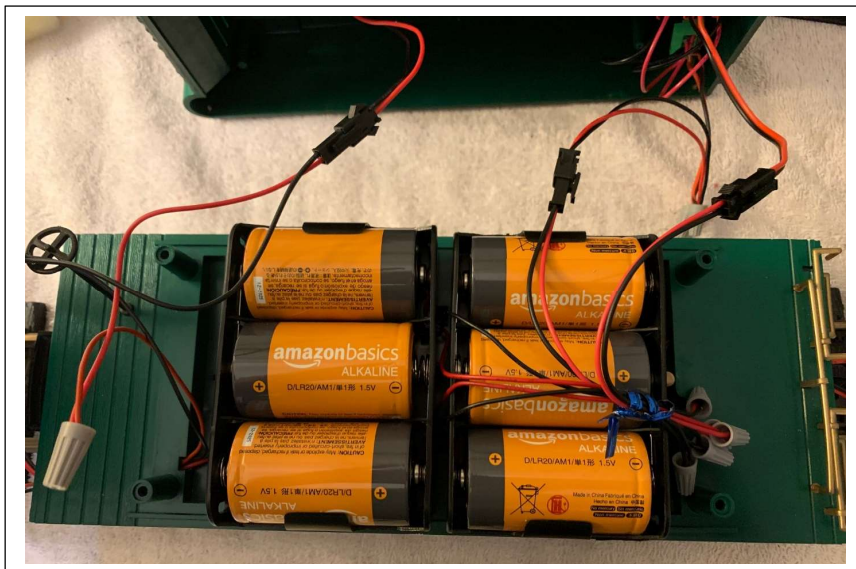
Six ordinary D-cells generate 9V of power to run the locomotive for about five hours
