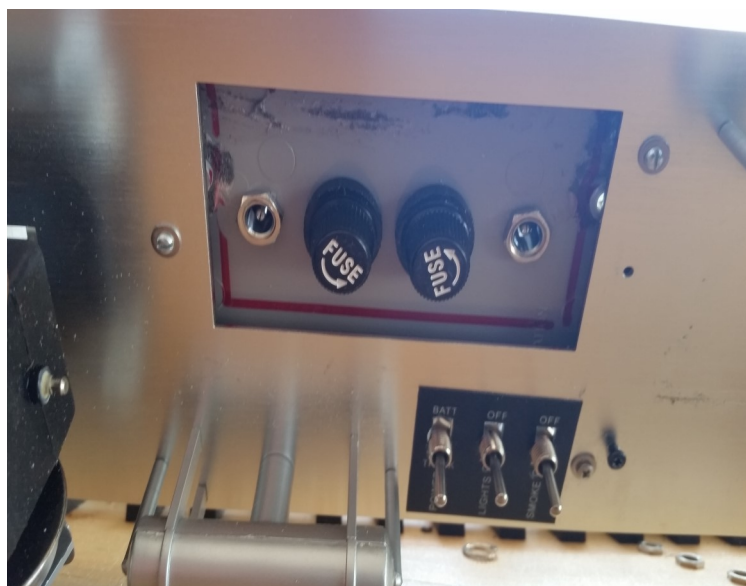
6. Underside of RDC showing switches, fuses and the charging jacks.
